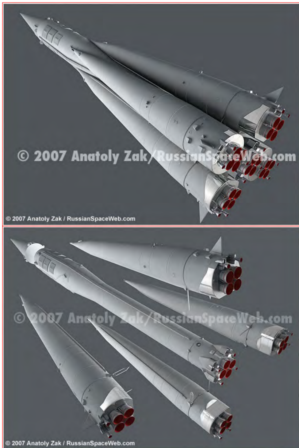
Figure 15P-6 Two-Stage R-7 Rocket Modified for Sputnik-1
