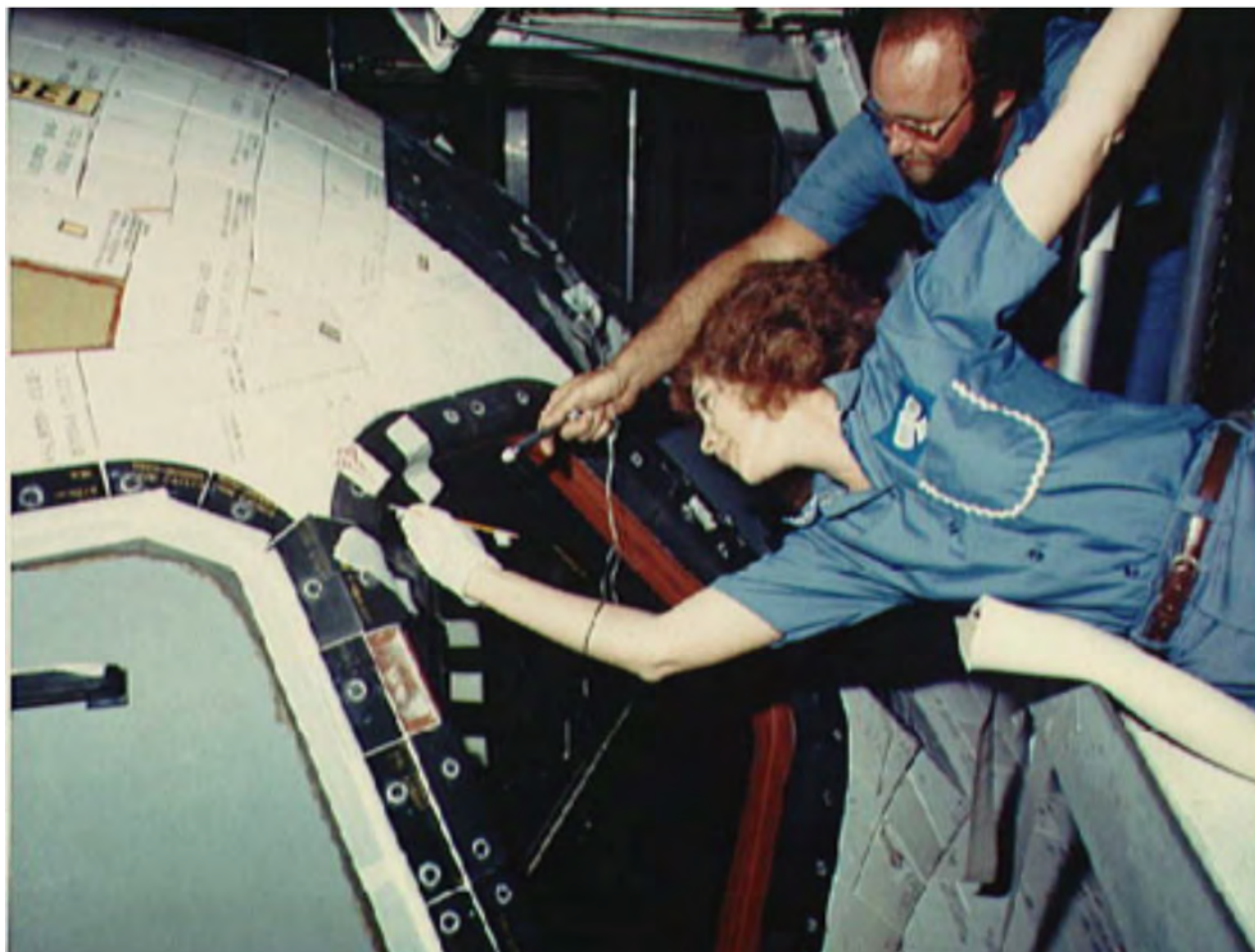
Figure 17O-4 Repairing TPS on Columbia
