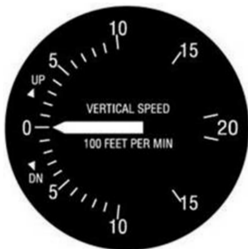
Figure 17B-3 Vertical Speed Indicator Parts
